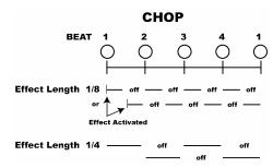
section then turn off for a section. This is important because you can reverse the sections that are off and on by activating the effect in the other section. If you deactivate the effect then turn it on again it remembers the last set parameter.
